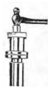
Fig. 8. Press Small Bearing Bearing on Shaft
